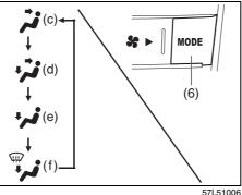
Push the "MODE" switch (6) to change among the following functions. The indication of the selected mode appears on the display. If the "AUTO" switch (9) is pushed, the air flow will vary automatically as the climate control system maintains the selected temperature.
